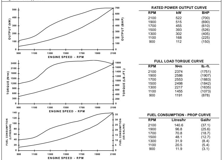
Rating Conditions: Ratings are based upon ISO 8665 and SAE J1228 reference conditions; air pressure of 100 kPa [29.612 in. Hg], air temperature 25°C [77°F], and 30% relative humidity. Power is rated in accordance with IMCI procedures. Member NMMA.
