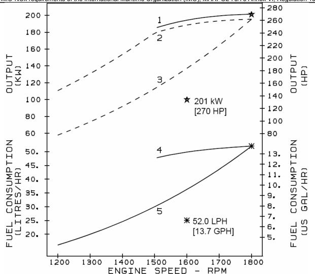
Rating Conditions:Ratings are based upon ISO 8665 and SAE J1228 reference conditions; air pressure of 100kPa [29.612 in.Hg] air temperature 25°C [77°F] and 30% relative humidity.Power is rated in accordance with IMCI prodedures.
